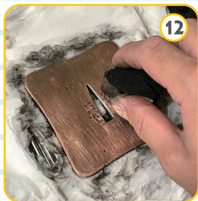
Polishing the surface and dipping in water mixed with finely grated daikon radish
