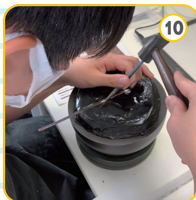
A long and thin billet is carved in the same way, and then stretched flat
