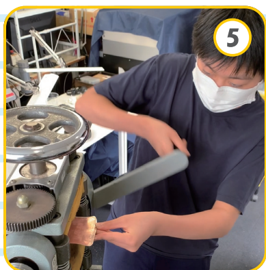
Repeating of stretching Tsuba by using a roller machine
