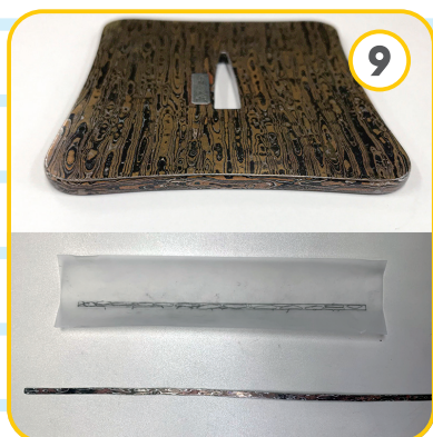
The “fukurin” in which the outer circumference is also made of Mokume Gane
