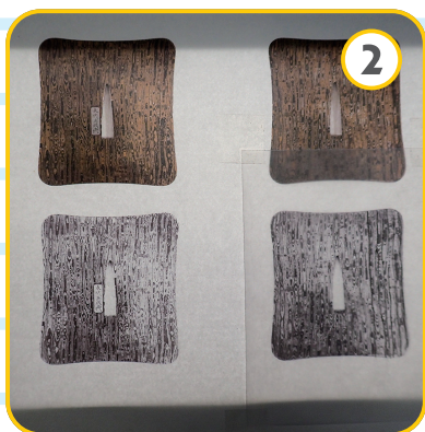
Transcribing the patterns of Tsuba so as to make the pattern on the base metal
